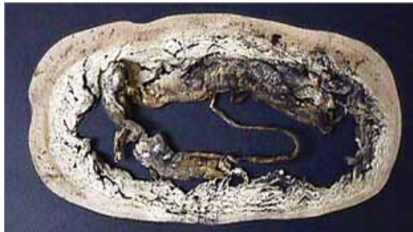
Figure 6.4a Deformation of a Spiral Wound Stainless Steel-PTFE Gasket Due to EO Permeation and Polymerization
