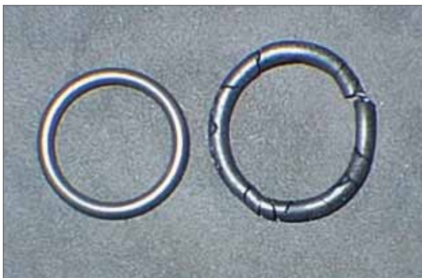
Figure 6.9 Butyl Rubber O-Ring Before and After Exposure to EO for 30 days
