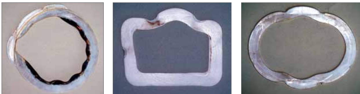
Figure 6.2 PTFE Gasket Failures in EO Service Due to Cold Flow
