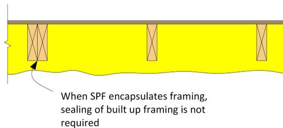
2. The SPF layer needs to completely encapsulate the interior UVA space so there are no gaps in the insulation or airtightness. In practical terms, this means that SPF must extend down and connect to the air barrier for above-grade walls such that discontinuities do not exist at eaves and projecting roof assemblies. (See Figure 3.2)
