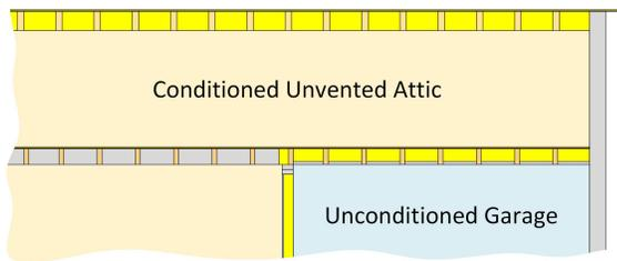
vapour barrier film behind drywall, or a Vapour Barrier primer on the interior drywall. (Note, the Vapour Barrier should not be applied on the attic floor as Vapour Barrier protection is needed directly in the insulated assembly which is now at the roofline.) Medium-density SPF meets code-compliant levels of vapour control to be classed as a vapour barrier at thicknesses over 50 mm (2.0 in.) so a supplemental Vapour Barrier is typically not required when MD SPF is used.
