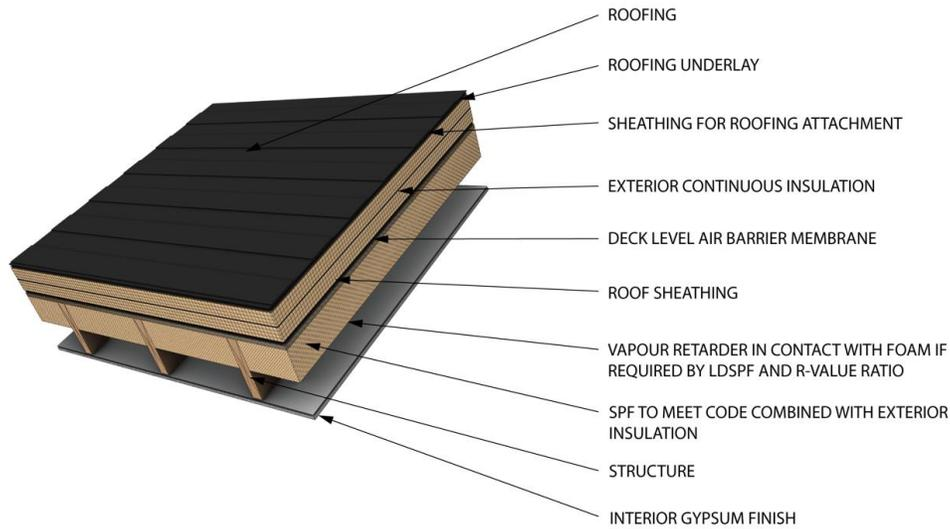
*Figure 8 : Roof assembly with exterior insulation and MDSPF*
