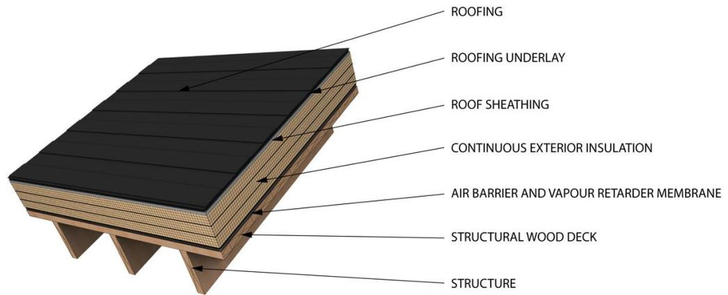
Figure 4 : Exterior insulated sloped roof assembly
