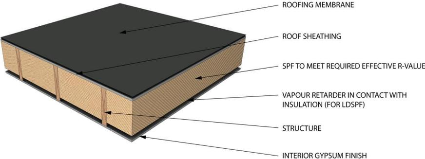
Figure 7 : SPF insulated flat roof
