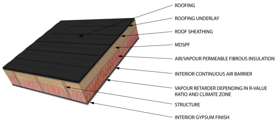
*Figure 10 : Hybrid roof assembly combination of air impermeable exterior MDSPF insulation installed against the interior of the roof sheathing and air/vapour permeable fibrous insulation to the interior of the spray foam.*
