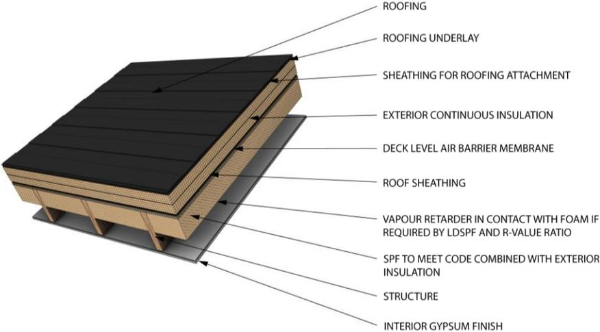
Figure 6 : SPF insulated sloped roof assembly
