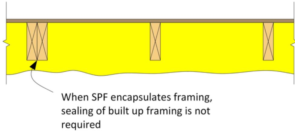
Figure 11 : Framing embedded in SPF should be encapsulated when possible to ensure air barrier continuity around the roof framing. (credit image to SFC<sup>3</sup>)
