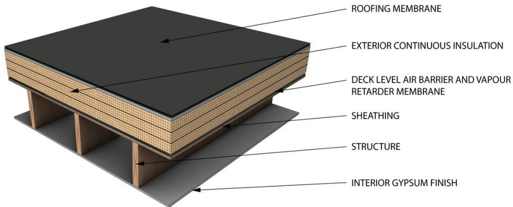
Figure 5 : Exterior insulated low slope (flat roof) assembly
