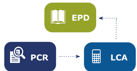
Figure 3. Product Category Rules (PCR) dictate the completion of a valid material or product life cycle assessment (LCA) and environmental product declaration (EPD).
