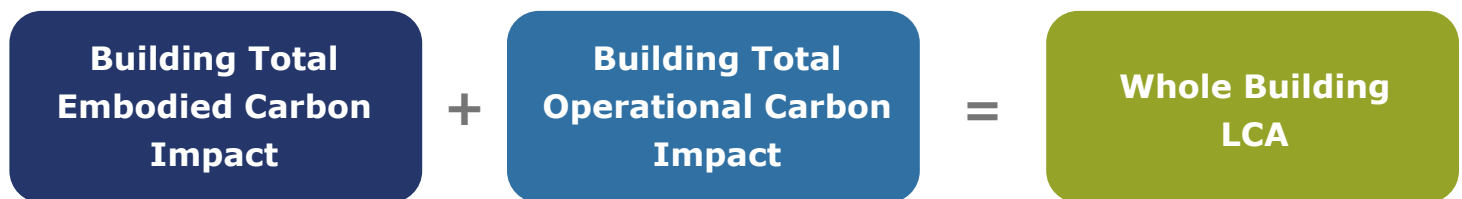
Figure 1. Whole building life cycle assessment evaluates the net GHG emissions and emissions savings attributed to a building's summed embodied carbon impact and operational carbon impact.
