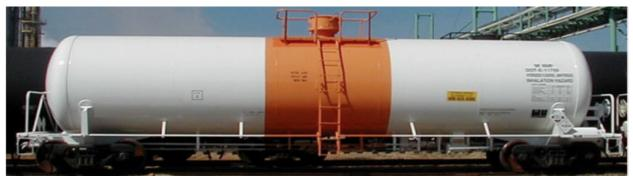
AHF is typically shipped 80-90 net tons, 23,000 U.S. gallon shell full, non-insulated tank cars designed according to the Association of American Railroads (AAR) "Manual of Standards and Recommended Practices, Specifications for Tank Cars." AHF tank cars are painted white and have a "safety orange" center band.
