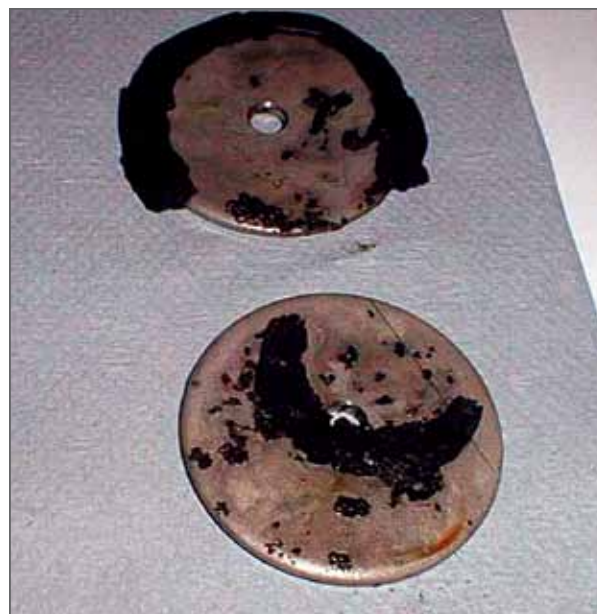
Figure 6.11 Example of Severely Degraded O-ring in High Temperature EO-water Service
