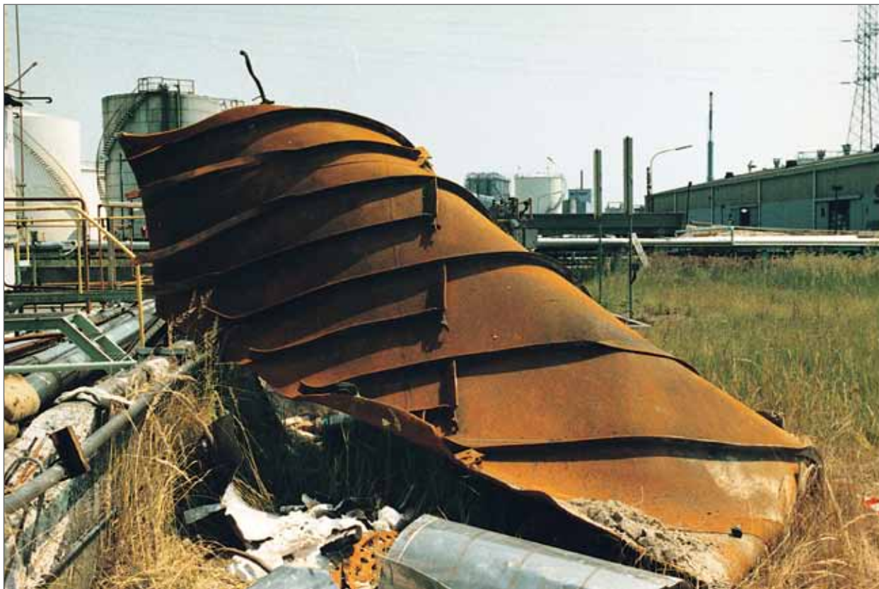
Figure 5.15 Piece of Ethylene Oxide Distillation Column Wall Turned Inside Out by Explosion
