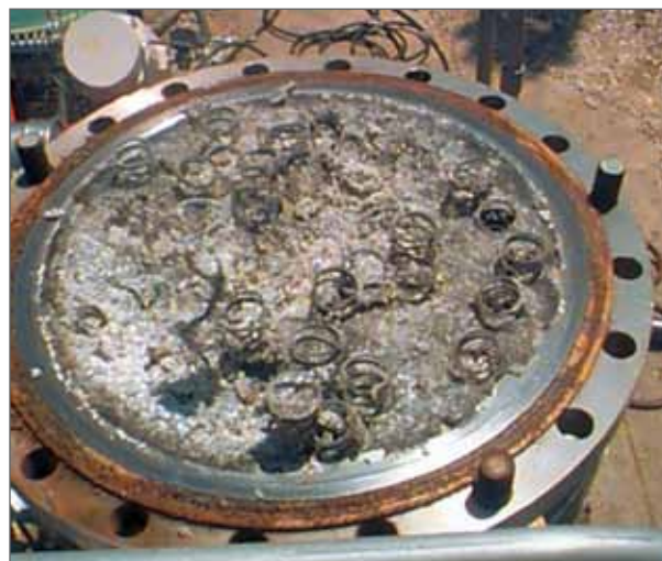
Figure 5.21 Filter Case after Runaway Polymerization
