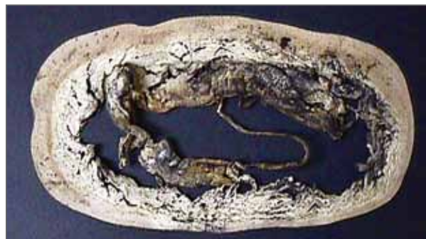
Figure 6.4a Deformation of a Spiral Wound Stainless Steel-PTFE Gasket Due to EO Permeation and Polymerization
