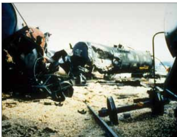
Figure 5.8 Damage to Other Railcars from Ethylene Oxide Railcar Explosion
