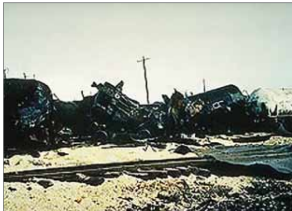
Figure 5.8 Damage to Other Railcars from Ethylene Oxide Railcar Explosion
