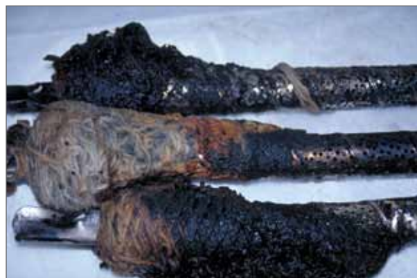
Figure 5.23 Filter Case after Runaway Polymerization
