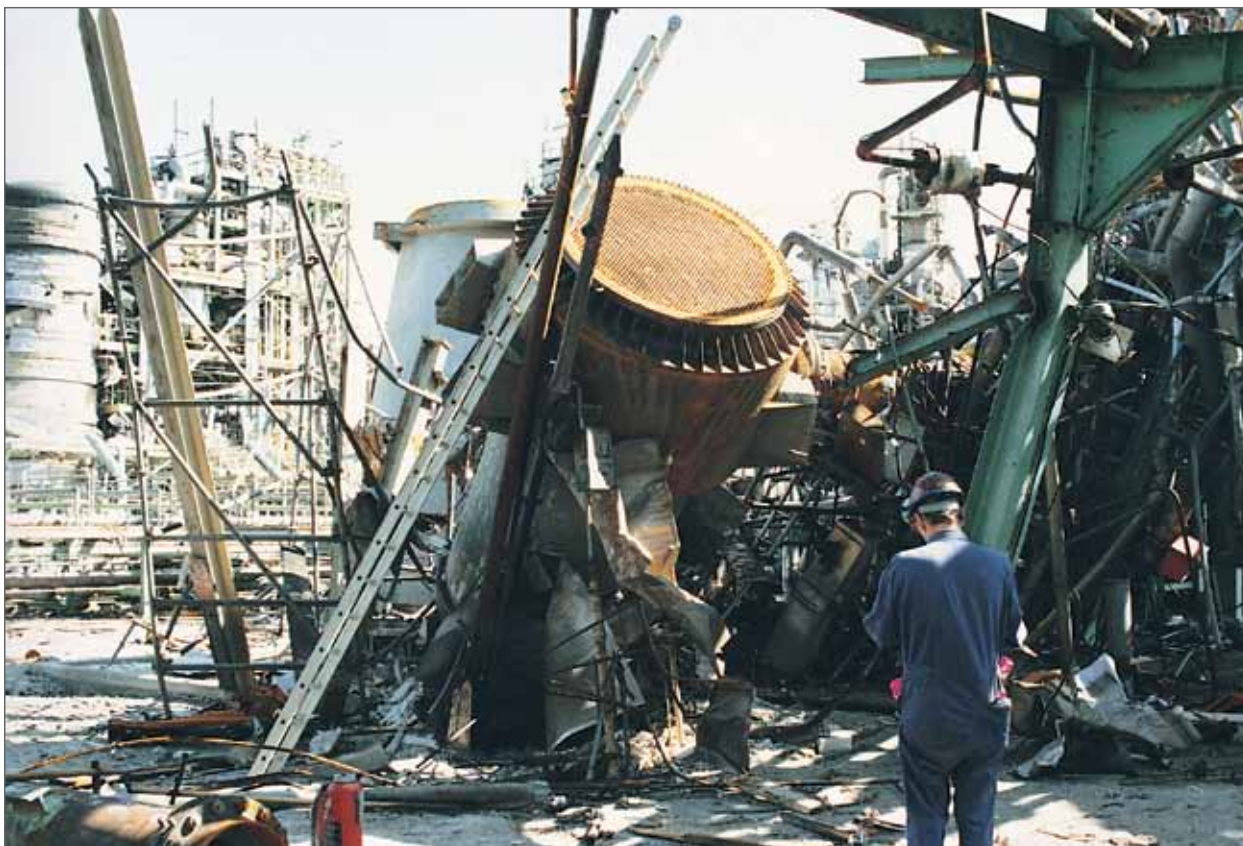
Figure 5.12 Ethylene Oxide Distillation Column Reboiler after Explosion
