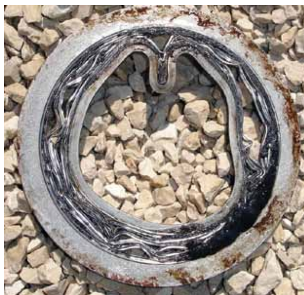
Figure 6.4b Deformation of a Spiral Wound Stainless Steel-PTFE Gasket
