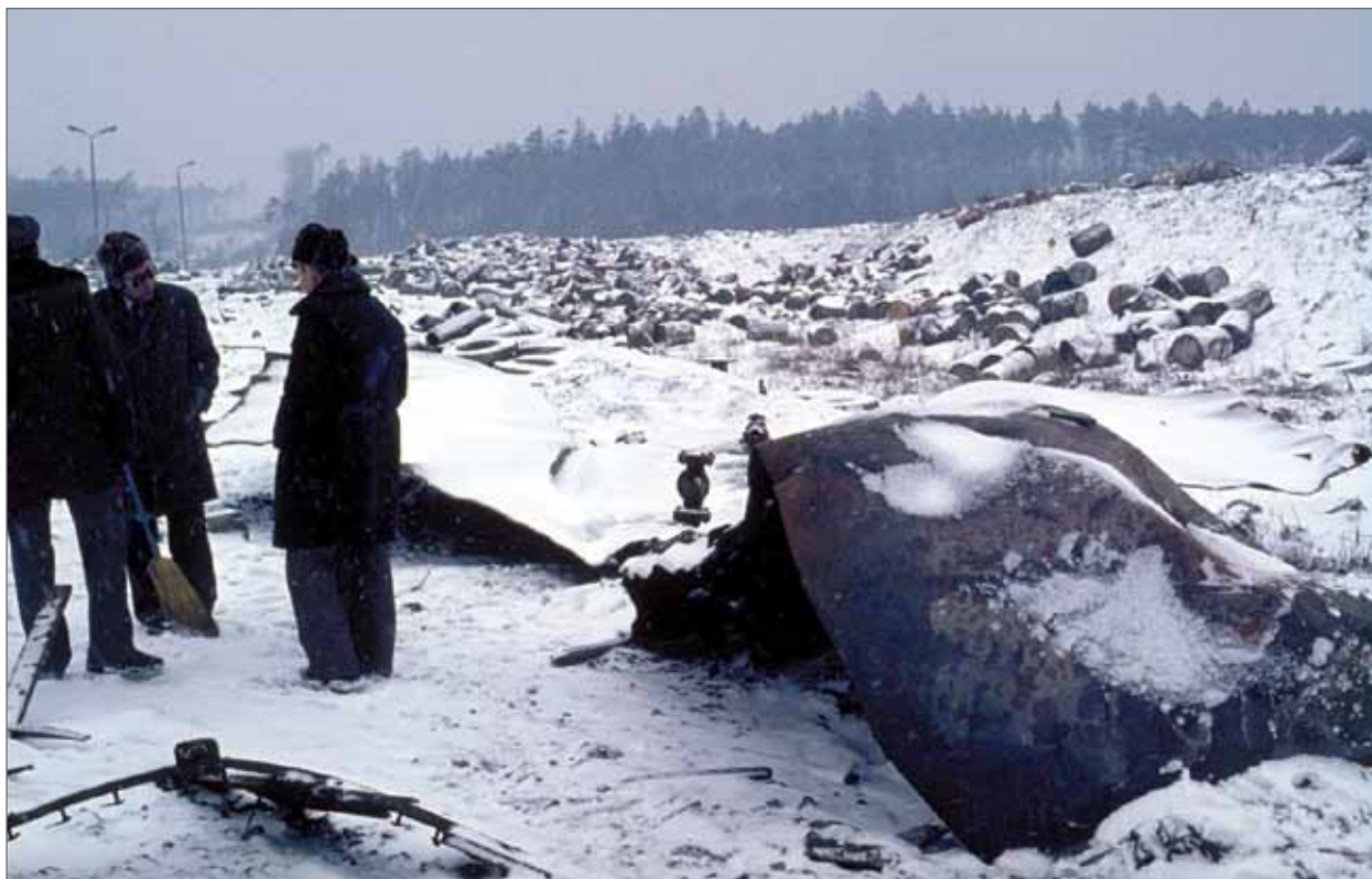
Figure 5.9 Remnants of Railcar (after EO explosion caused by contamination with ammonia)
