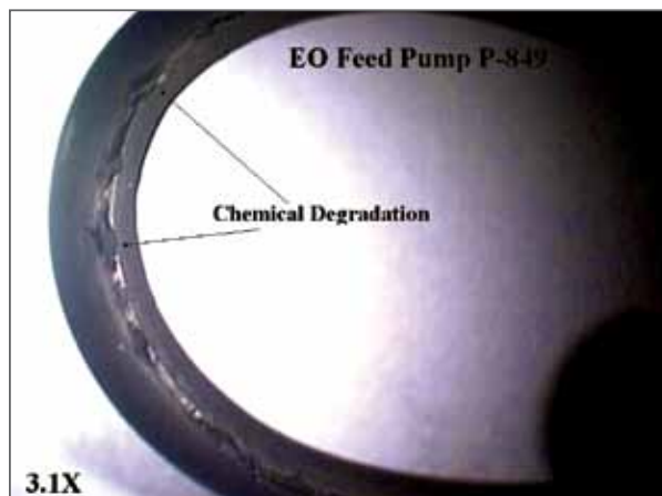
Figure 6.10 Example of Degraded O-ring Attacked by EO
