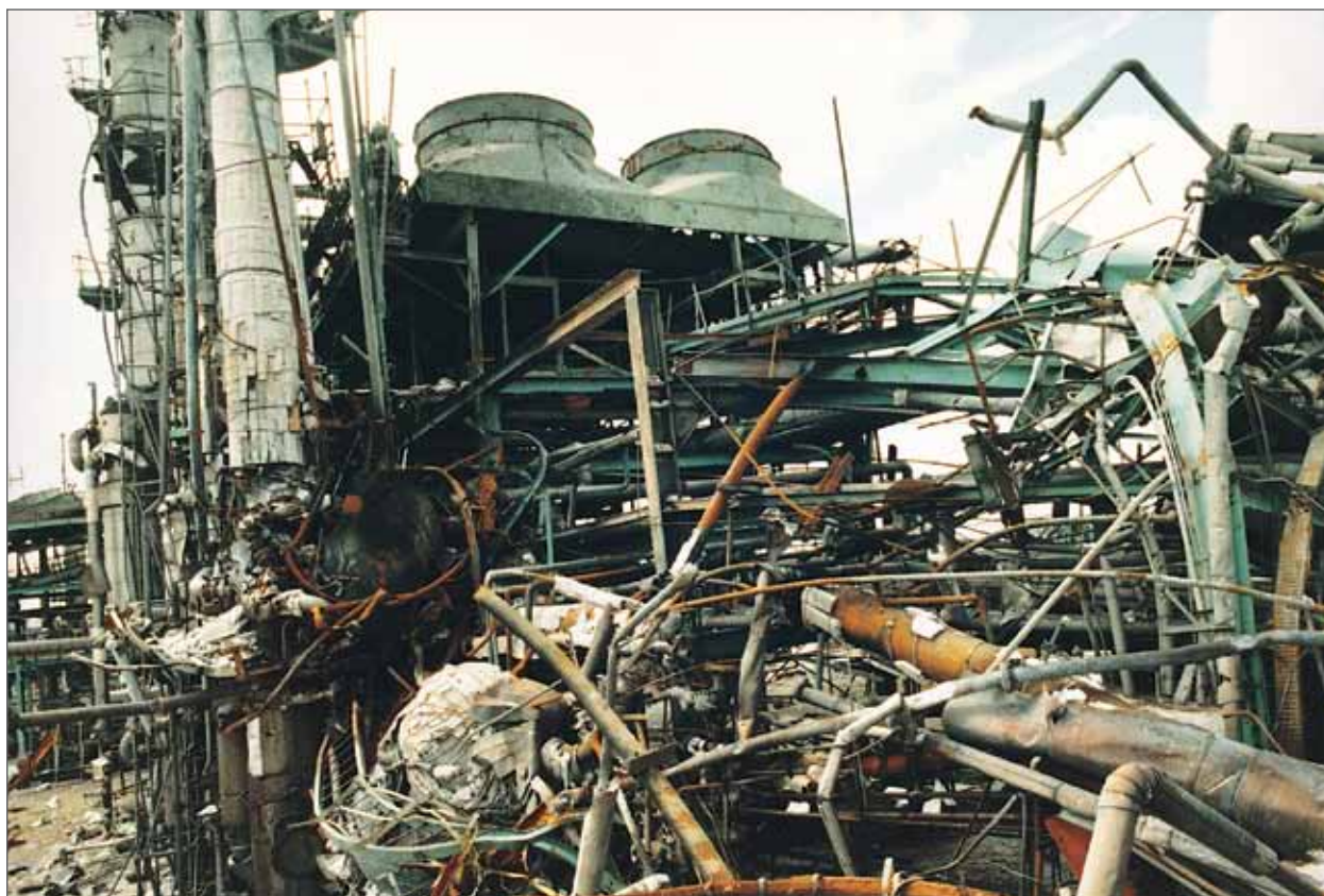
Figure 5.14 Remnants of Base of Ethylene Oxide Distillation Column after Explosion
