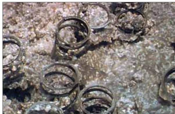
Figure 5.22 Filter Case after Runaway Polymerization
