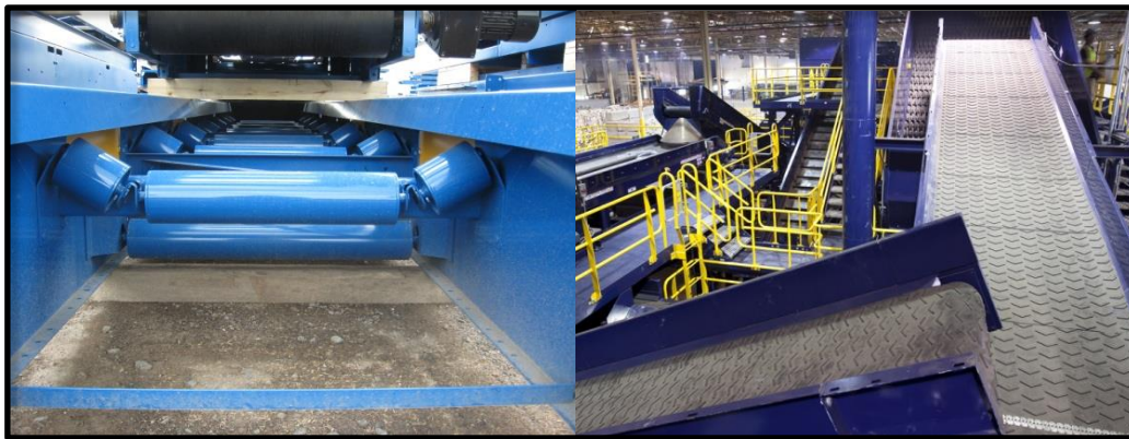
Figure 6 The Following are Examples of An Idler Conveyor (no belt) and Slider Conveyors
