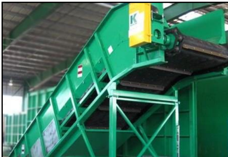
Figure 7 The Following is An Example of a Chain Belt Conveyor
