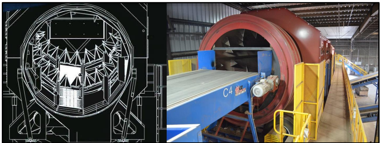
Figure 3 The Following is An Example of a Trommel with Bag Opening Cutters
