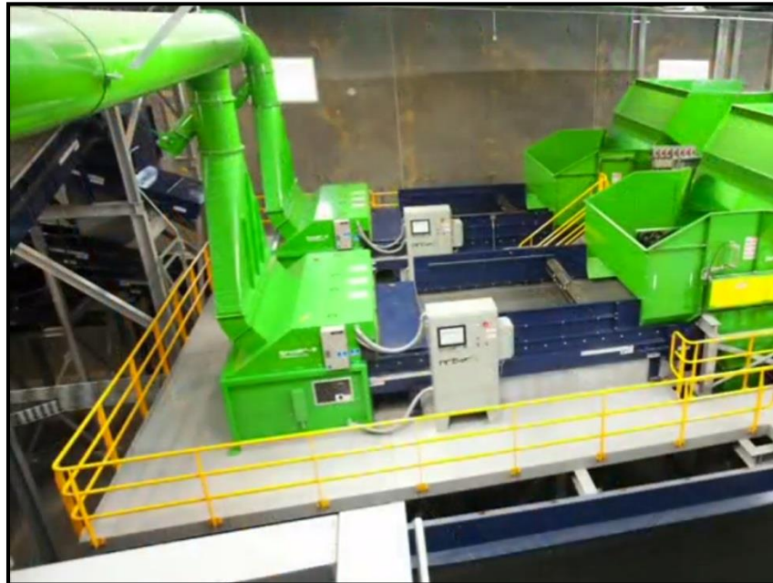
Figure 5 The Following is An Example of Film Optical Units with Pneumatic Transfer
