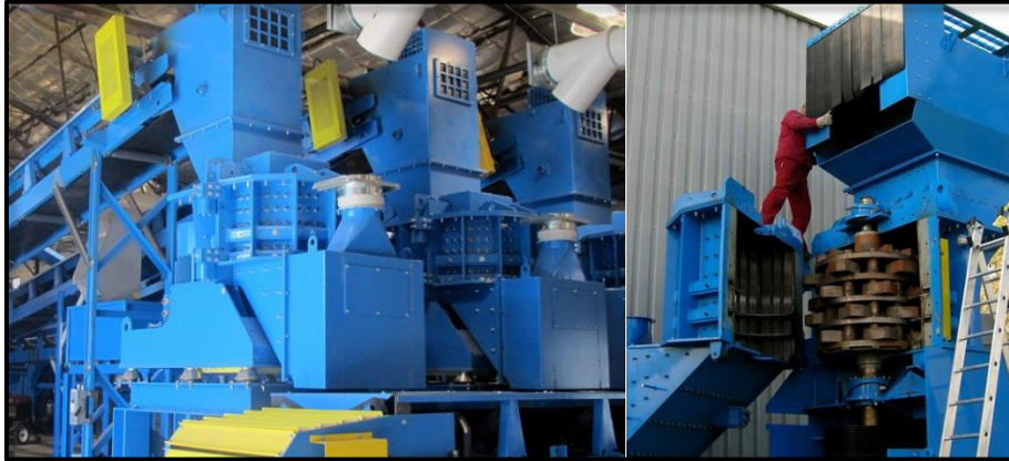
Figure 11 The Following are Examples of Vertical Hammermills
