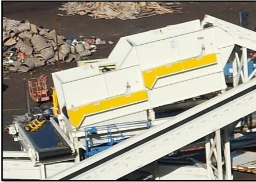
Figure 2 The Following is An Example of a Declining Screen
