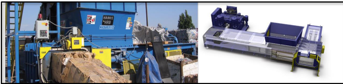
Figure 28 The Following are Examples of Dual Ram Balers
