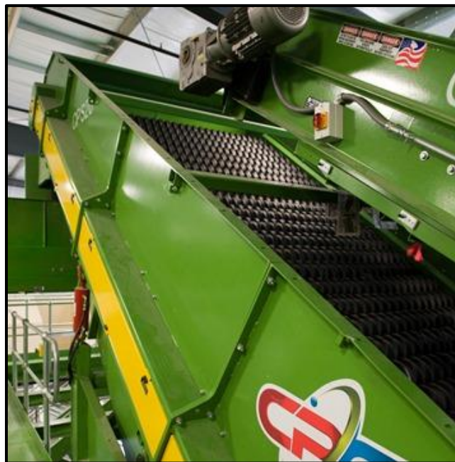
Figure 17 The Following is An Example of a 2D/3D Screen
